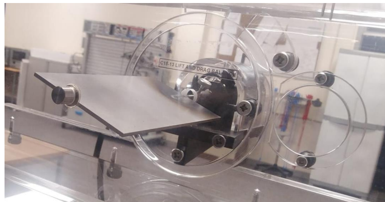
Figure 1. Solar PV panel sample examined in the wind tunnel.
