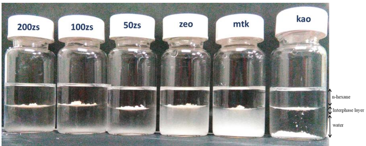
Figure 6 Dispersion behaviour of samples in hexane-water mixture
