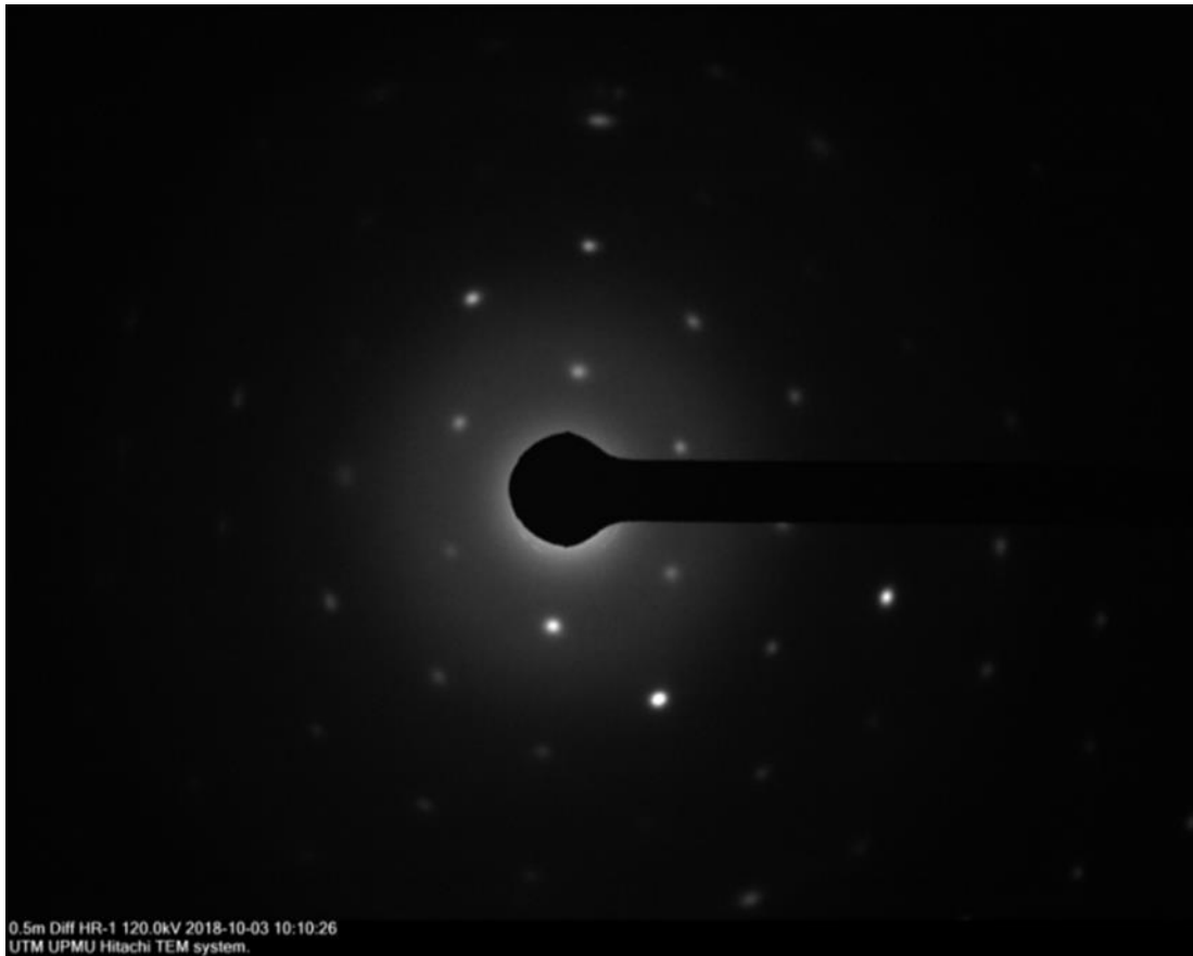
Figure 5 Selected area electron diffraction (SAED) pattern of ZEO-STREP
