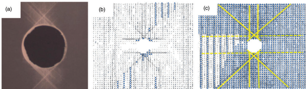
Figure 16. Damage zones associated with [45^\circ/0^\circ/-45^\circ/90^\circ]_{2s} IM7/8552 CFRP composite specimens: (a) X-Ray experimental result, 41 (b) damage zone represented by cracks at strain of 0.58%, (c) damage zone represented by cracks at strain of 0.73%.
