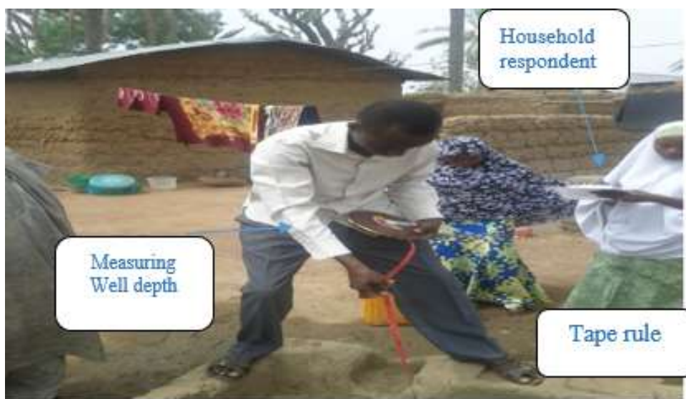
Figure 6.3 Field measurement of Hand-dug well depth using tape rule
