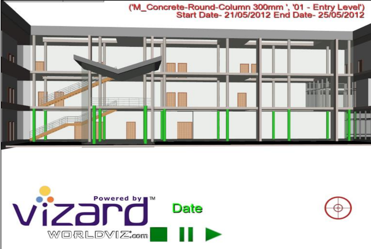
Figure 0-4 All columns on 1st storey selected - no date assigned
