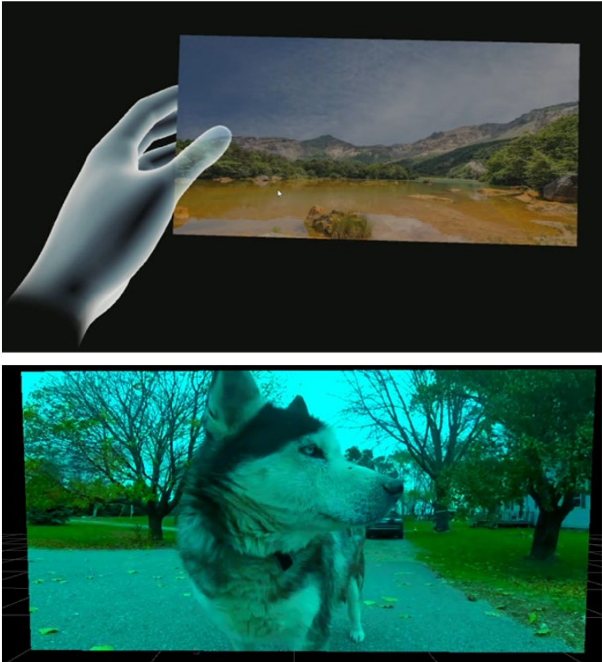
Fig. 7. (Top) A video shrunk to the user's hand in our prototype; (Bottom) A video with colors adjusted to compensate for Protanopia color-blindness.
