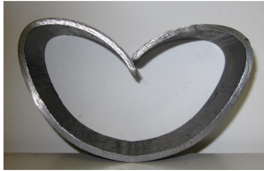
Figure 24: The final collapse profile of specimen with a point load application.
