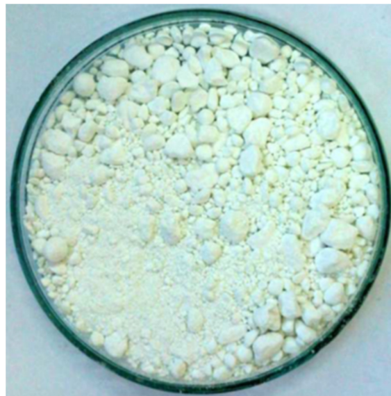
Figure 2. LDPE powder (PE-T) recovered from Tetra Pak ® packaging after precipitation, separation, and drying.
