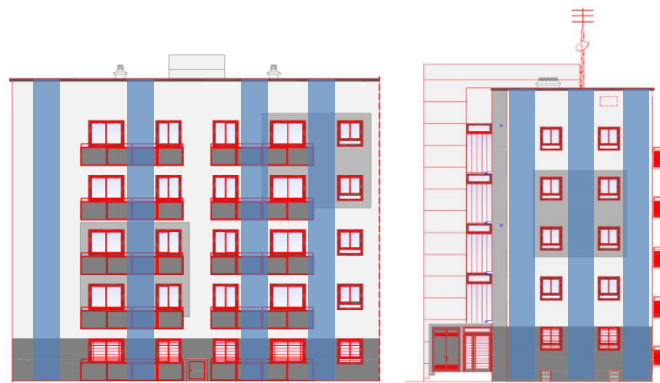
Figure 7. South West (left) and South East (right) façades of the target building incorporating vertical panels shown in blue
