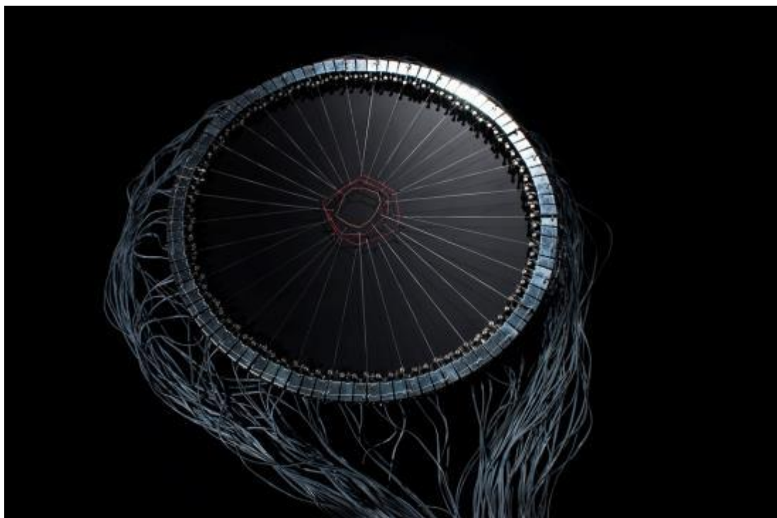
Fig.10 The Conversation (2009) © Ralf Baecker A ring of sensor-actuators autonomously maintain the tension of the three bands that form a surface around a void in the centre of the device.
