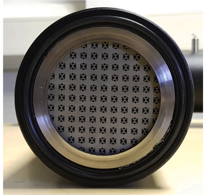
Fig. 3. 3D printed titanium MPP mounted in the impedance tube.
