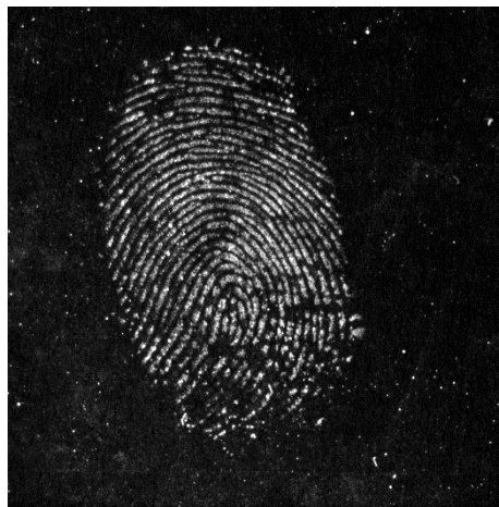
Figure 1. A latent fingerprint on a polymer banknote that has been treated with fp Natural 1™ fingerprint powder and visualised under 600-650nm illumination with 715nm long-pass camera filter using a Foster + Freeman Crime-lite Imager.
