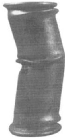
Figure 8: Global bending in axially crushed foam filled circular tubes [59]
