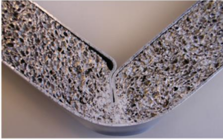
Figure 10: Deformation mode of foam-filled tubes under bending loading [71]
