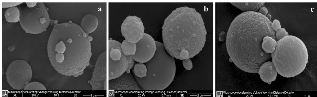
Fig. 6 Scanning electron microscope image of microparticle (5000 x): a CZ (chitosan zein microparticles with no active compound), b CZ-R (chitosan-zein microparticles loaded with rutin), c CZ-VDR (chitosan zein microparticles loaded with vitamin D 3 and rutin). The white bar in each image represents 2 µm
