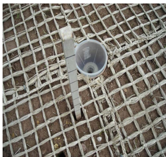
Plate 4. Plan view of a scale and splash collector.
