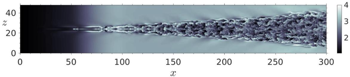
**Figure 3:** Instantaneous temperature field at  $y=1.4$  within the boundary layer ( $D=1.2$ )
