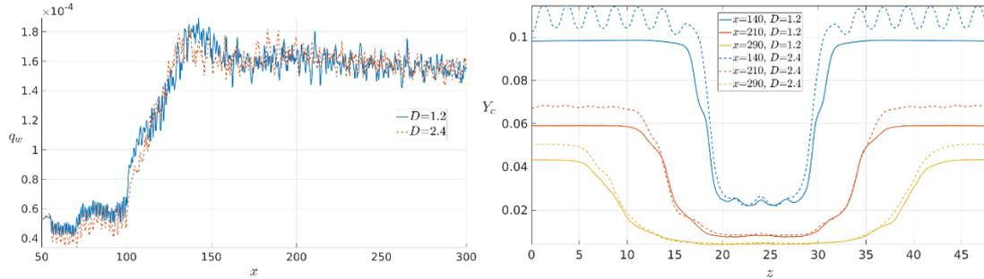
**Figure 5:** Time-averaged spanwise-averaged wall heat flux within the turbulent wedge (left) and time-averaged  $z$ -wise coolant concentrations at different  $x$  stations downstream of the injection region (right)
