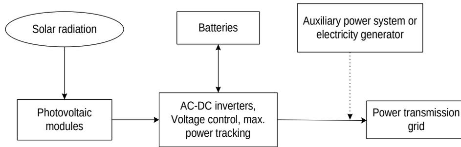
**Fig. 1** Schematic diagram of a large-scale grid-connected PV system with energy storage (Koroneos et al. 2006a).
