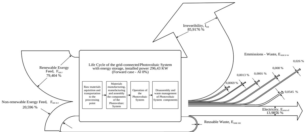
**Fig. 6** Sankey diagram for Life Cycle of the PV System, where the total exergy inflow is expressed in terms of Non-Renewable and Renewable Exergy Feed. (Forward case - AI 0%).
