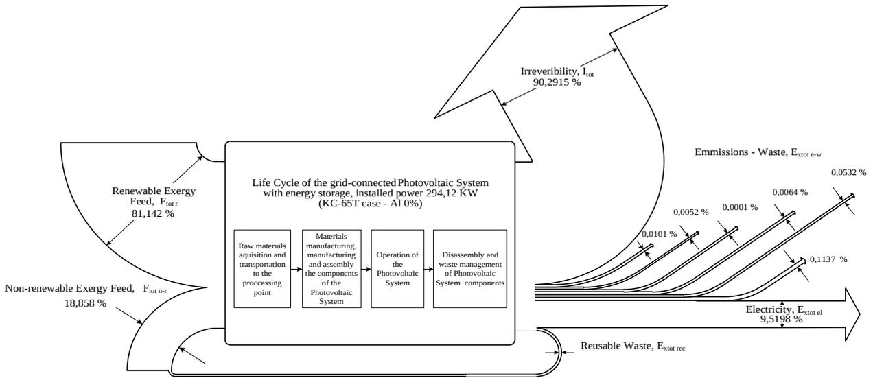
**Fig. 4** Sankey diagram for Life Cycle of the PV System, where the total exergy inflow is expressed in terms of Non-Renewable and Renewable Exergy Feed (KC-65T case - AI 0%).
