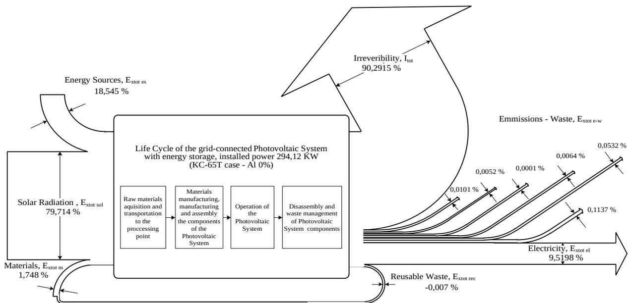
Fig. 3 Sankey diagram for Life Cycle of the PV System. (KC-65T case - Al 0%).
