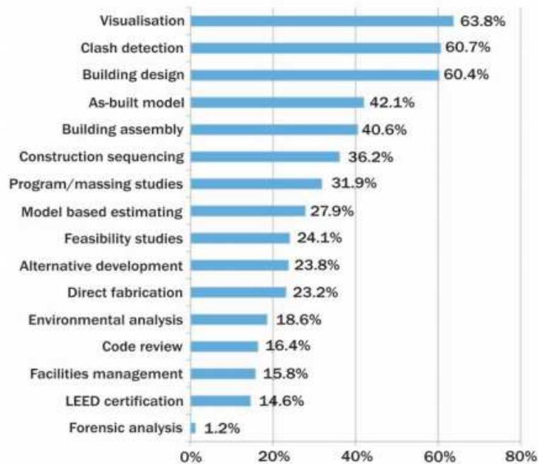
Figure 1- Most popular tasks using BIM (Gerber and Rice 2010)
