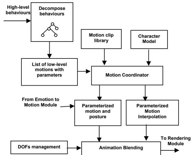
Figure 2 Architecture and functionalities of the motion generation module
